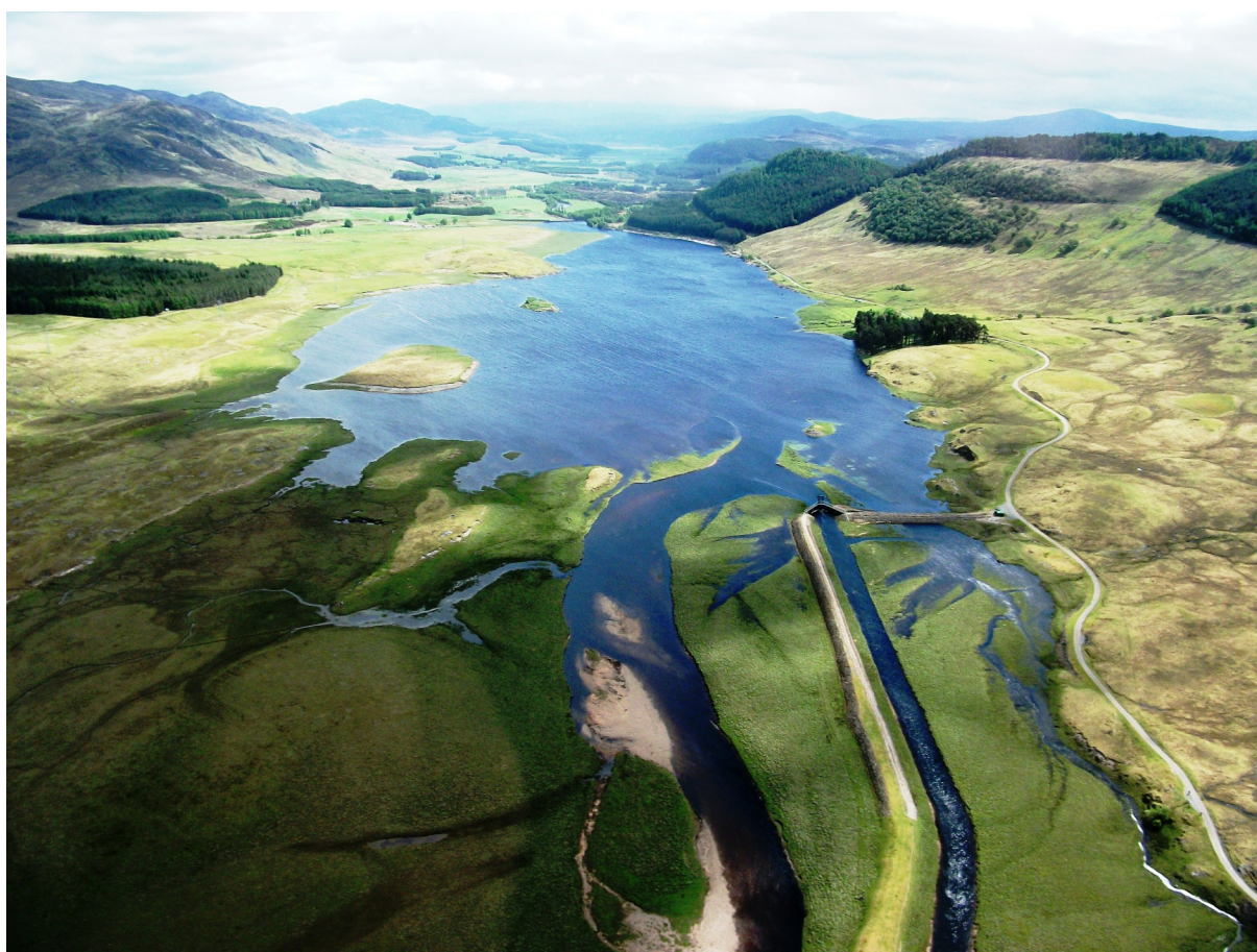
Above : An aerial view of the River Spey as it enters the reservoir above Spey Dam. The off-take and the Crunachden Cut, down which water is diverted to Fort William via Loch Laggan, is clearly visible to the right of the River Spey. (Photo: Roger Knight)
