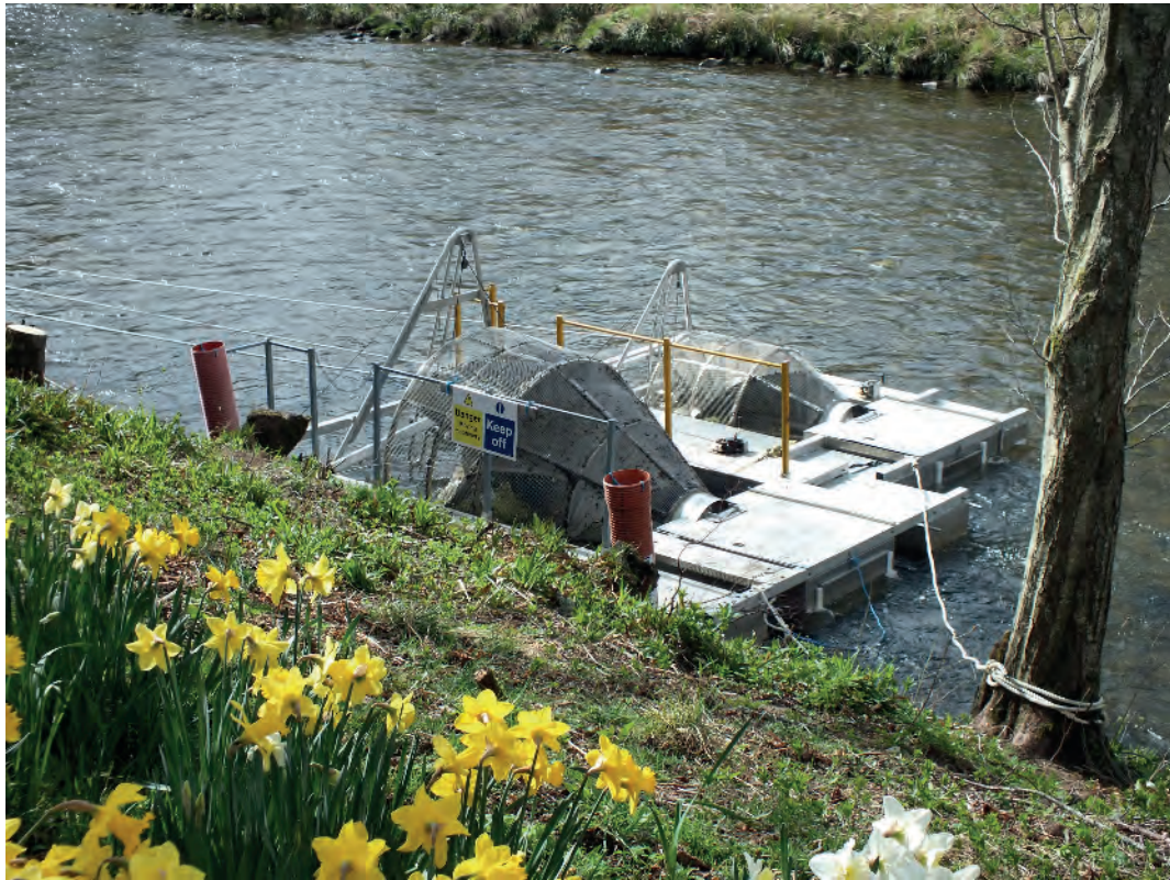
Above: The Twin Rotary Screw Traps in operation on the lower River Avon. (Photo: Brian Shaw).
