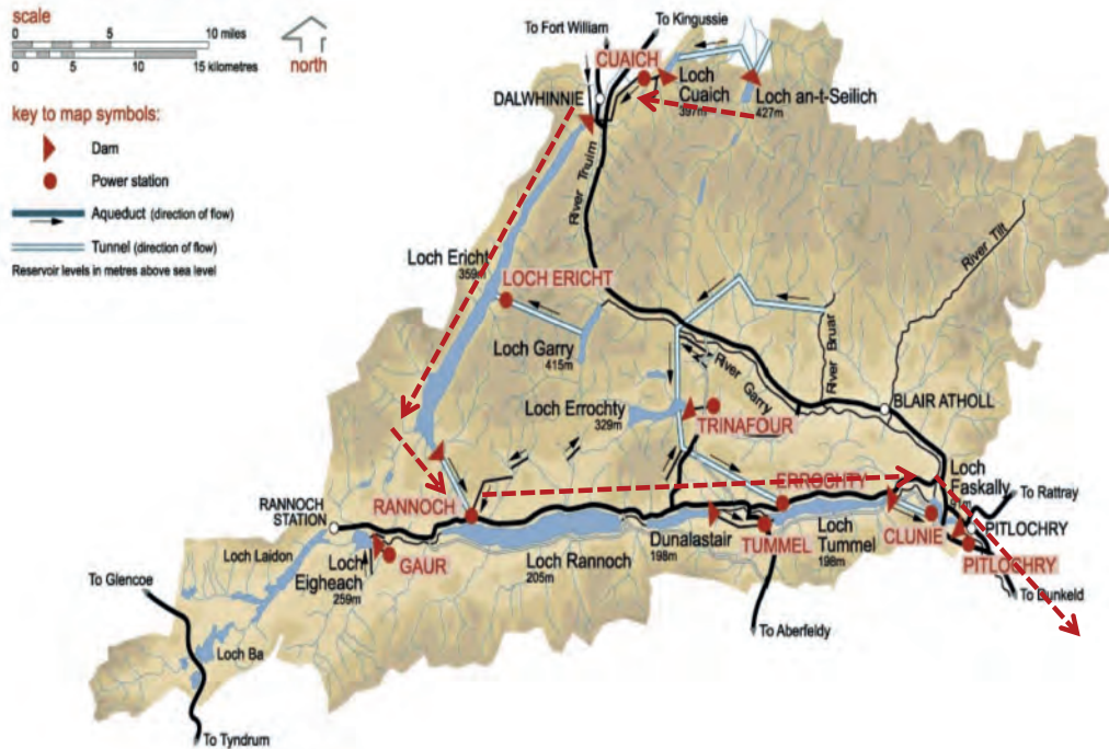
Figure 3: Scottish & Southern Energy's Tummel Scheme CAR Licence allows the diversion of water from the Spey Catchment into the Tay catchment. The red dotted line illustrates the current regime as water is taken from the Spey's upper tributaries, the Rivers Tromie and Truim, and transferred into the Tay catchment to pass through seven power-generating stations.
