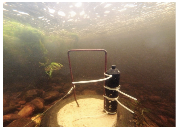
Above photo shows the Acoustic Tag used (Courtesy of Marine Scotland). Below photo shows one of the receivers in position in the River Spey.
